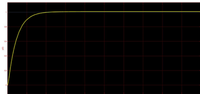
Fig. 18. The response of PID-Fuzzy Logic controller 5*5, 7*7 rules base.
